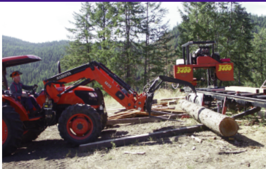
Bruce uses his Kubota tractor with log grapple to place a log on the mill's lifting arm. Once the log is in place, Bruce says that the arm easily lifts 30-in.-diameter by 24 ft. long larch and Douglas fir logs.
